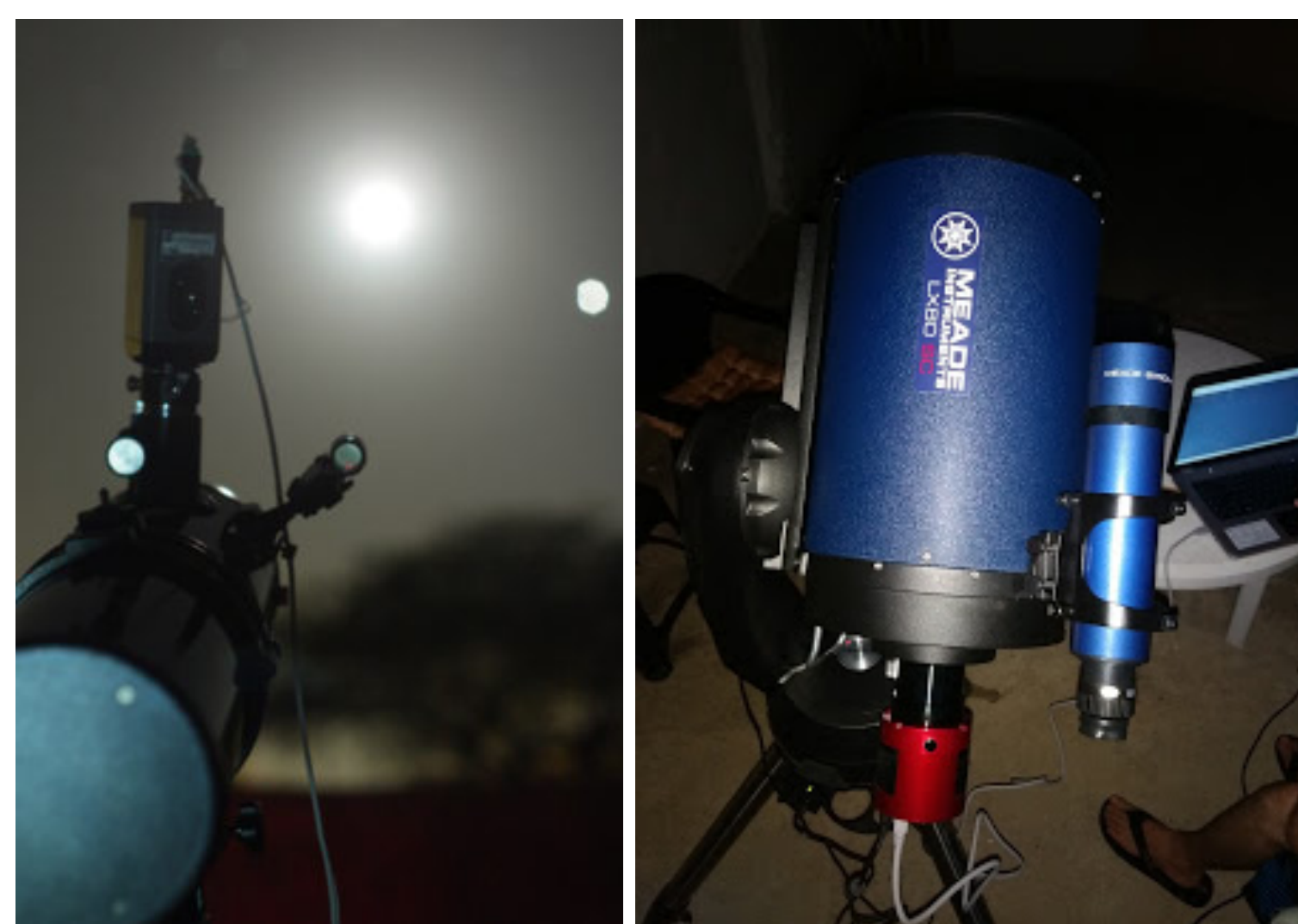
Figure 4: Setups used in Moon footage. Left: Skywatcher 130mm F5 + Samsung SCB 2000 camera. Right: Meade LX80 8" + ASI 1600 CCD
