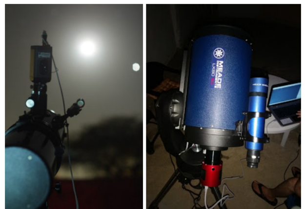
Figure 3 – Setups used in Moon footage. Left: Skywatcher 130mm F5 + Samsung SCB 2000 camera. Right: Meade LX80 8” + ASI 1600 CCD
